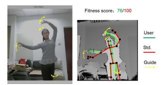
**Figure 3** The proposed Virtual Personal Trainer. The left is the user video captured by the camera of the Kinect. The right is the real time skeleton of the user (shown in green lines) and the matched standard skeleton (shown in red lines). The fitness score is shown above the skeleton in real time. The action correction guide in 3D space is shown in both the user video and the skeleton video.
